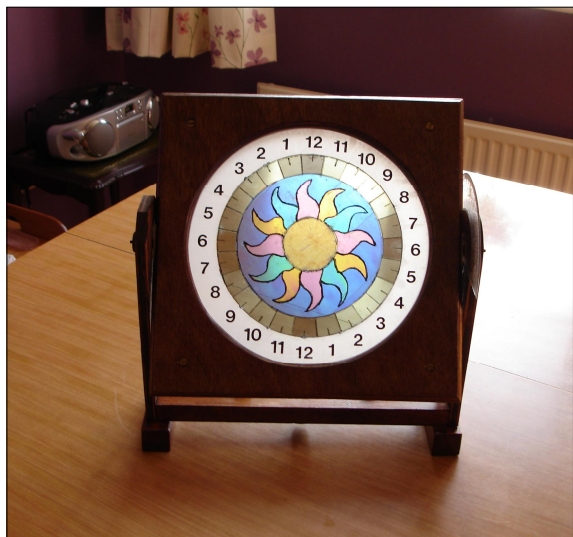
Fig. 8 (above). Dial viewed indoors by light partially polarized horizontally.
