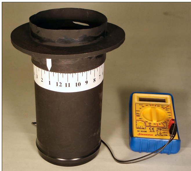
Fig. 2. The polarization sundial/sky polarimeter.
