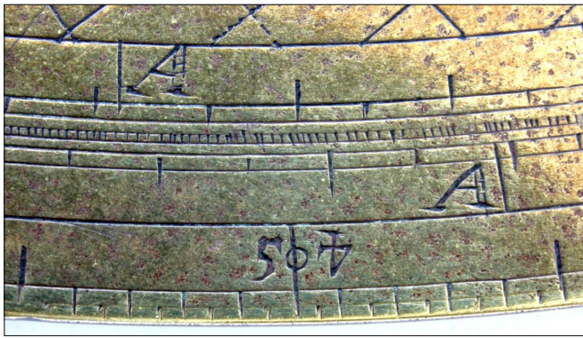
Fig. 13. Outer degree scale of the quadrant showing 50° and the inverted 40° using a common 0.
