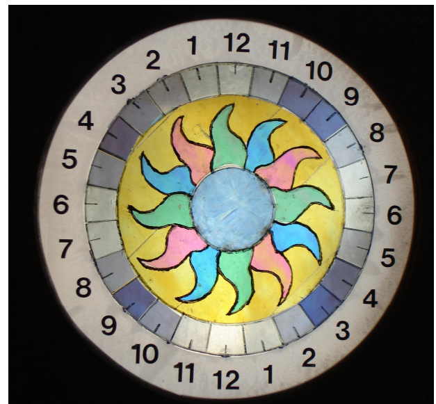
Fig. 13. Dial illuminated by light partially polarized in a vertical plane, indoors.
